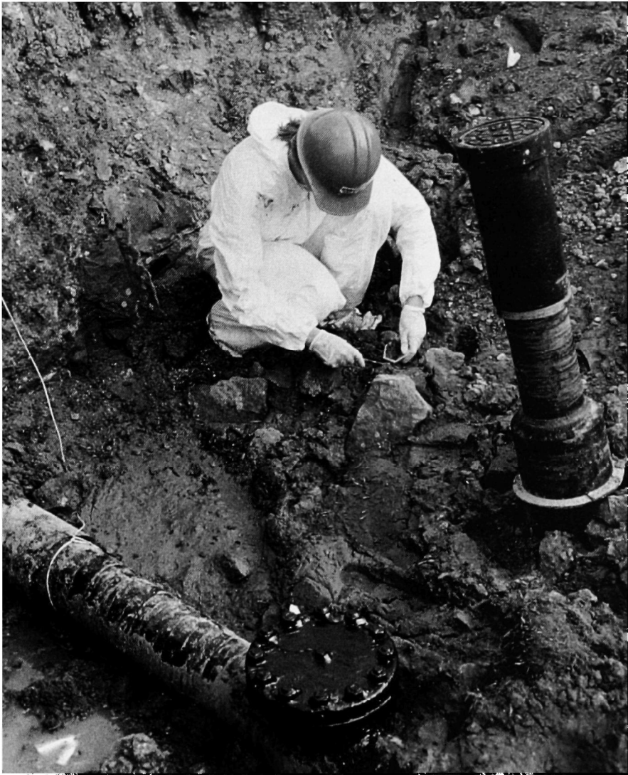
Technician collects soil samples for immunoassay testing.
