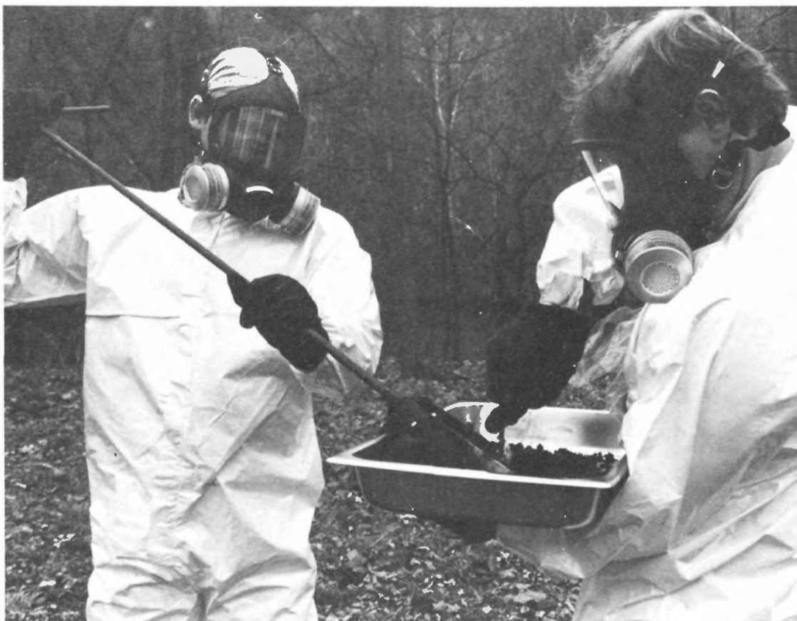
Collecting soil samples to measure possible dioxin contamination. Even though EPA is reassessing its original dioxin cancer risk estimates, dioxin is still considered to be a highly toxic cancer-linked compound. A modern, affluent society offers many benefits, but also presents risks.
