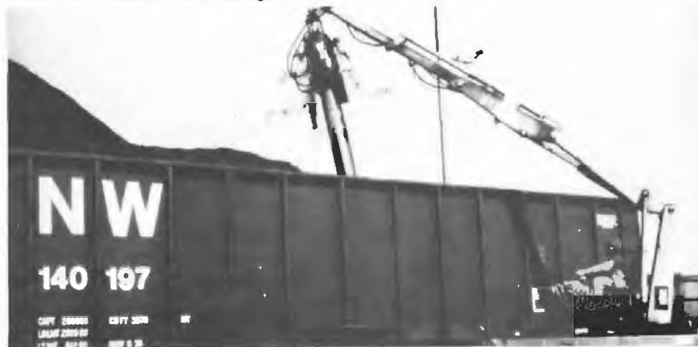
Coal sampling by Potomac Electric Power Company at its generating plant in Alexandria, Va. Sulfur, ash, and capacity to produce heat are measured.
