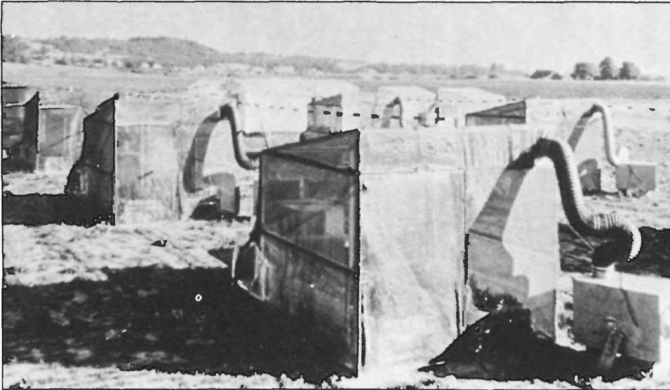
Plastic tents enclose test crops on EPA's 4 1/2-acre farm, where effects of polluted air on field crops and trees are measured.
